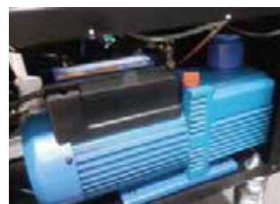
Strong Vacuum pump 142 l / min double stage
